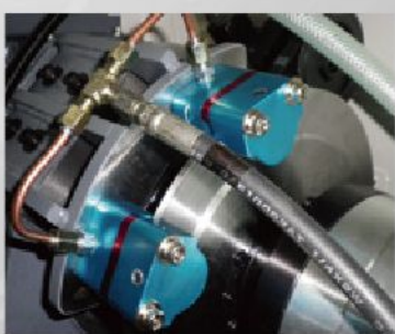
C軸功能-碟剎裝置 C-axis function (Disc brake device)
