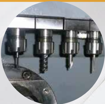
側銑裝置 Cross side live tooling device
