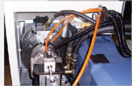
▲ 副主軸吹氣及推料裝置 Air-blowing and finished parts ejector device for Sub-spindle
