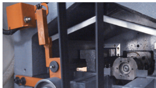
主軸皮帶檢知裝置 Belt break detection device of spindle
