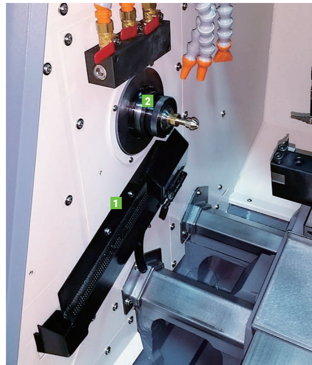
櫛式刀具板 Gang type tool plate
